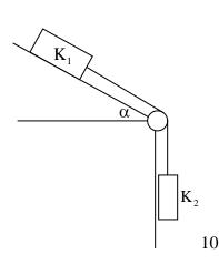
$$\begin{split} a &= g \sin \alpha = ... \approx 5, 6 \tfrac{m}{s^2} \\ v^2 - v_0^2 &= 2 a s_1 \quad \Rightarrow \quad v^2 = 2 a s_1 + v_0^2 = 2 s_1 g \sin \alpha + v_0^2 \quad \Rightarrow \quad v = \sqrt{2 s_1 g \sin \alpha + v_0^2} = ... \approx 5, 9 \tfrac{m}{s} \end{split}$$
