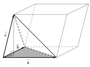
$$V_{\text{3-seitige Pyramide}} = \frac{1}{6} \cdot \left| \left( \vec{a} \times \vec{b} \right) \circ \vec{c} \right| = \frac{1}{6} \cdot \left| \det \left( \vec{a}, \, \vec{b}, \, \vec{c} \right) \right|$$
